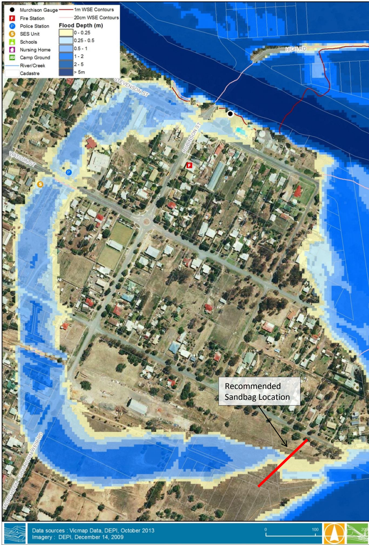
Figure 4-6 Recommended Sandbagging Location for Extreme Flood Events
